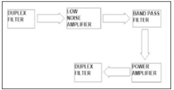
Fig. 3. Block Diagram of Signal Amplifier
